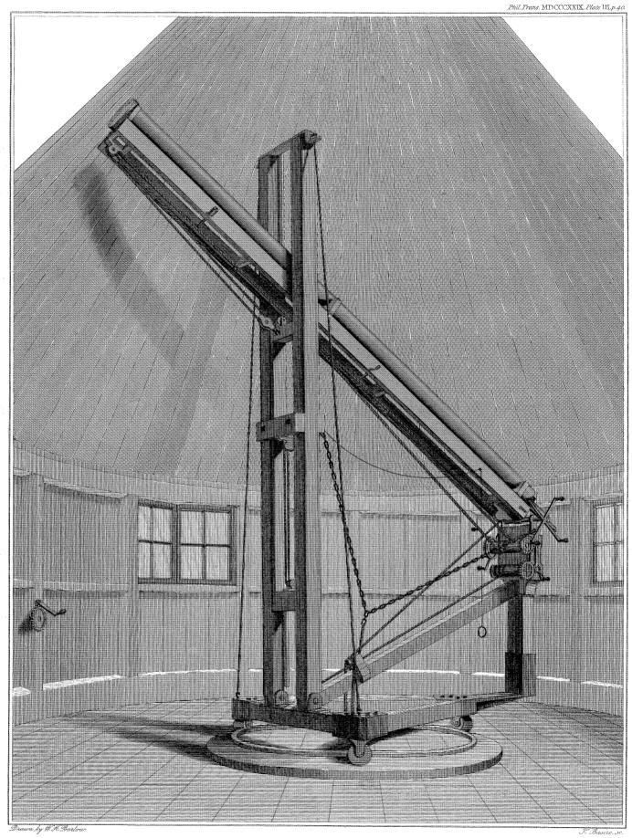
The front socket is different from the others, as it forms one piece with an upright socket which carries a strong oaken stancheon, to the upper part of which the machinery described below is attached. This stancheon having to support a great part of the weight of the telescope, at least in some positions of the latter, is strongly braced back by an oaken beam to the opposite ledge of the triangular base.
